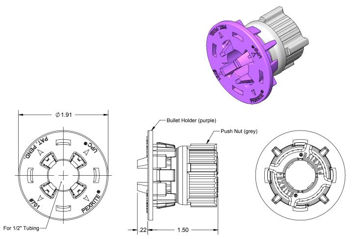
The PEXRITE® LOCK-n-LOAD<sup>™</sup> #701 is a clamp that mounts into our PEXRITE #103, #709, #110-R or #721 Series Bracket. This clamp requires no hardware to install and is designed to firmly grip fixture stub-outs such as bullets or similar 1/2" CTS tubing. The PEXRITE LOCK-n-LOAD #701 is for use with PEXRITE Brackets only.
