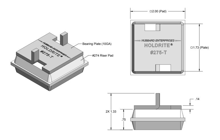
The HOLDRITE Silencer™ #275-T is an engineered sound and vibration riser pad with a steel bearing plate. Ideal for use in isolating riser clamps from noise and vibration transfer to the structure. Unique vertical tabs protect from incidental displacement.
