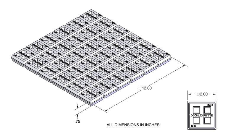
The HOLDRITE Riser Pad #274 individually measures 2" X 2" X 3/4", that comes in sheet of 36. These can be separated from the sheet using scissors or knife.
