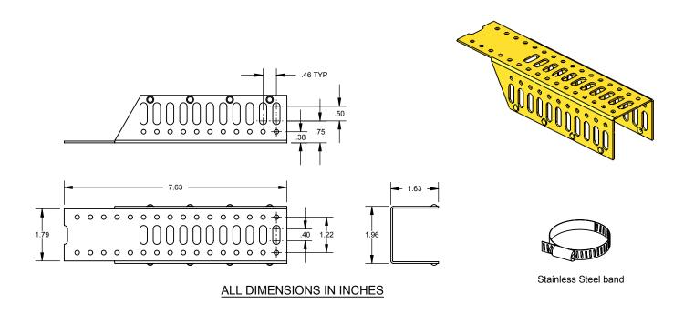
The HOLDRITE® #115 and #115-C (Copper-Bonded™) are steel brackets designed to position water supply lines off the vent or waste pipe in chase walls. Supports 1/2" through 2" pipes both vertically and horizontally. Packaged with self-locking stainless steel band, screws, metal clamps, and self-adhesive isolating felt. Excellent for pre-fab applications. Supports piping prior to wall framing. Heat the pipe, not the bracket when soldering the #115-C version.
