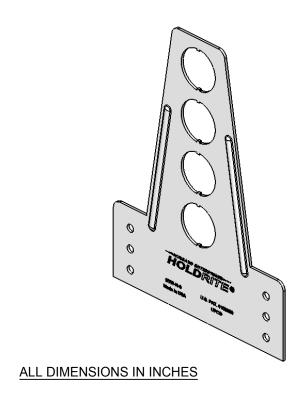
The LOCKRITE™ #609-N-6 is a 16 gage galvanized steel bracket with 1" hole on 1-1/4" centers. Ideal for toilets or hose bib stub-outs. Also serves as a nail plate. This bracket is designed to work exclusively with our glueable HOLDRITE® #604 (1/2") of #605 (3/4") inserts when installing CPVC tubing. Inserts snaps into bracket.
