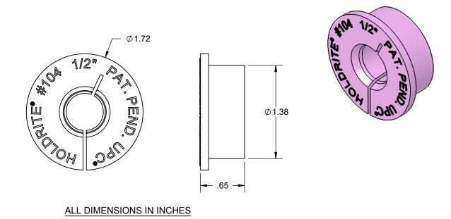
The HOLDRITE #104 insert is designed to work with HOLDRITE #103, #121, #709 and #125 series brackets. For Copper, PEX and CPVC tube.
