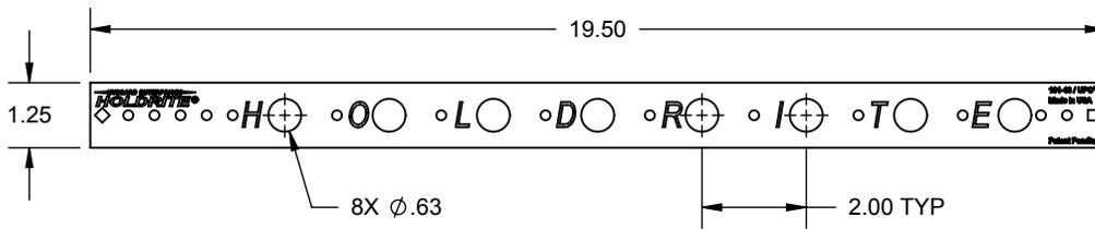
The HOLDRITE #101-18 is a Copper-Bonded™ steel bracket with 5/8" holes on 2" centers to support 1/2" copper tubing. The #101-18 position copper water supplies for sinks, water closets, and other fixtures. When soldering, heat the pipe, not the bracket.
