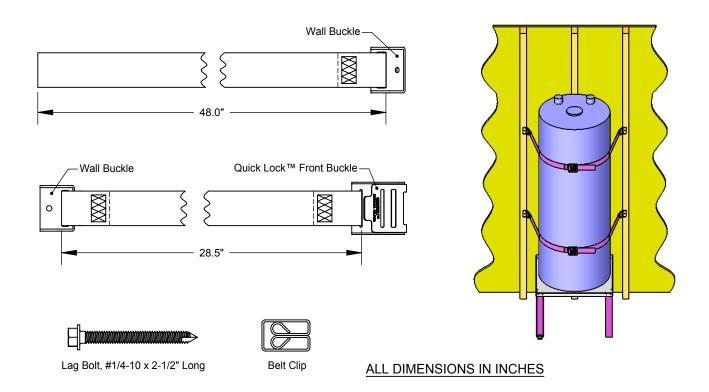
The QUICK BELT<sup>™</sup> #QB-50-F is a seismic/earthquake support system for water heaters up to 80 gallons in size. The system includes: (4) Straps, (4) Lag Bolts and (2) Belt Clips. The Quick Lock<sup>™</sup> system allows for secure locking of the strap from the front side of the water heater.
