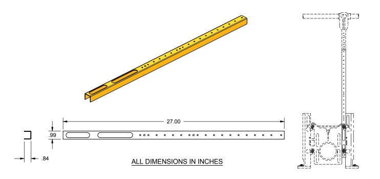
The HOLDRITE® #114-C-EXT is a Copper-Bonded™ steel bracket used to extend the flushometer rough-in height of the model #114-C, #114-CO and #114-CR an additional 8-1/2" through 24-1/2". The bracket mounts to the water closet carrier. Includes hardware for connection to the #114-C, #114-CO and #114-CR brackets.
