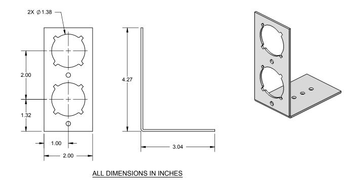
The PEXRITE® #709-L is a 14 gage galvanized steel bracket with 1-3/8" keyed holes providing an approximate 3" to 5" center line off of the attachment surface. Designed to work with our PEXRITE® #701 Clamp and #704 Insert. Ideal for lavatories, toilets and hose bibs. Compatible with HOLDRITE® #100 and #400 series inserts.
