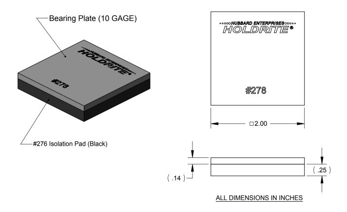
The HOLDRITE® Silencer™ #278 is an engineered sound and vibration isolation pad with a steel bearing plate. Ideal for use in isolating riser clamps and equipment bases from noise transfer to the structure.
