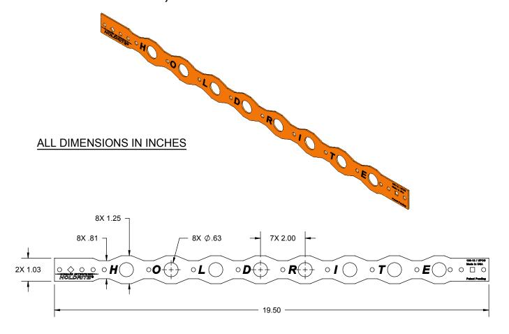
The HOLDRITE #100-18 is a Copper-Bonded™ steel bracket with 5/8" holes on 2" centers to support 1/2" copper tubing. The #100-18 positions copper water supplies for sinks, water closets, and other fixtures. When soldering, heat the pipe, not the bracket.
