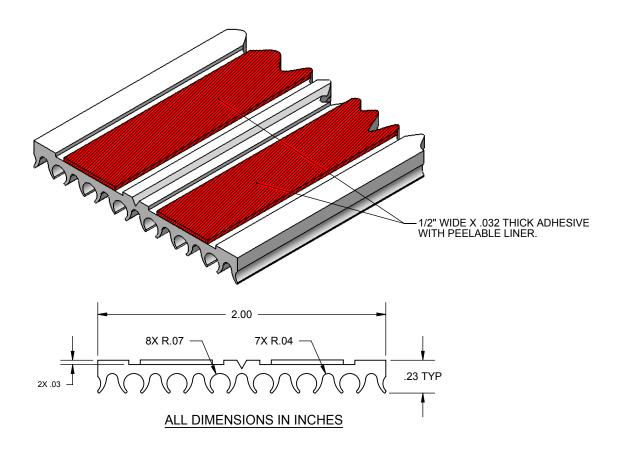
The HOLDRITE® Silencer™ #271 is an engineered sound isolation lining with many versatile applications for use in minimizing noise transfer with plumbing and piping systems. This 2" wide strip comes in 25' rolls and can easily be cut down the center at 1" width. The self-adhesive strips provide grip to piping or hangers. Excellent for use in isolating against sound or dissimilar metal contact in hangers or through framing components.
