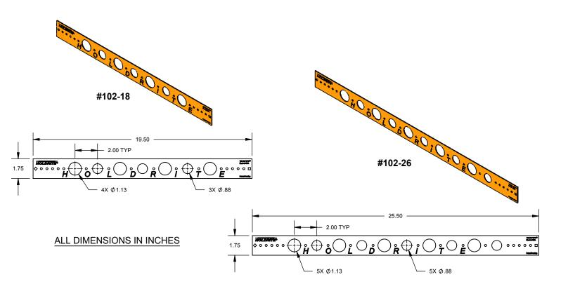
The HOLDRITE #102-18 and #102-26 are Copper-Bonded<sup>™</sup> steel brackets with holes to support 3/4" and 1" copper tubing. Used to support stub-outs for hot water tanks, urinals and other fixtures. When soldering, heat the pipe, not the bracket.
