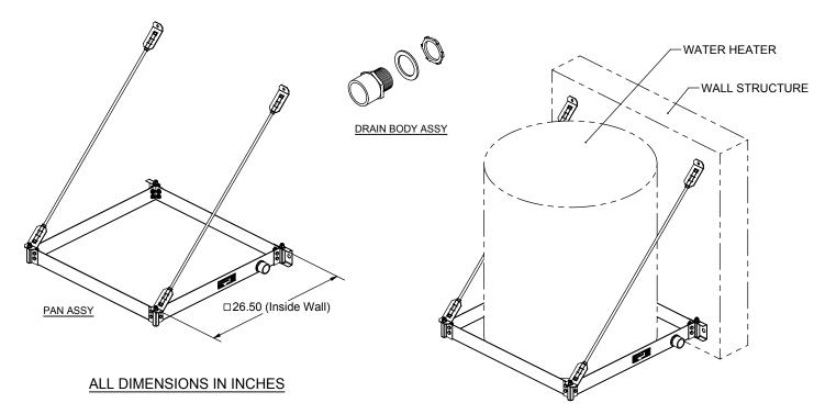
The Wall Mounted Equipment Platform is engineered to support water heaters up to 50 gallons (or other equipment up to 600 pounds total weight) mounted to a wall. This item also serves as a drain pan.
