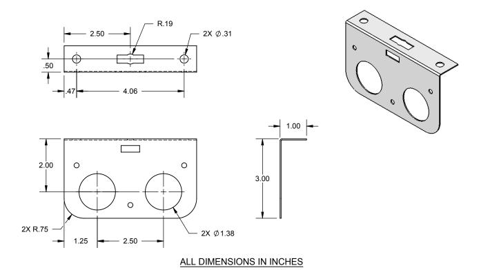
The HOLDRITE® #121-D is a 20 gage galvanized steel bracket that supports dual lines of 1/2", 3/4" or 1" Copper, PEX or CPVC tubing at 2" center line height. The hole pattern on the  $90^{\circ}$  base allows for attachment to any flat surface. The bracket can also be suspended by 3/8" threaded rod.
