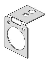
The HOLDRITE® #121-R is a 18 gage galvanized steel bracket with a 1-1/4" center line which will position 1/2", 3/4" or 1" Copper, PEX or CPVC for securing singe tubing to any flat surface. The bracket can also be suspended by 1/4" or 3/8" threaded rod.
