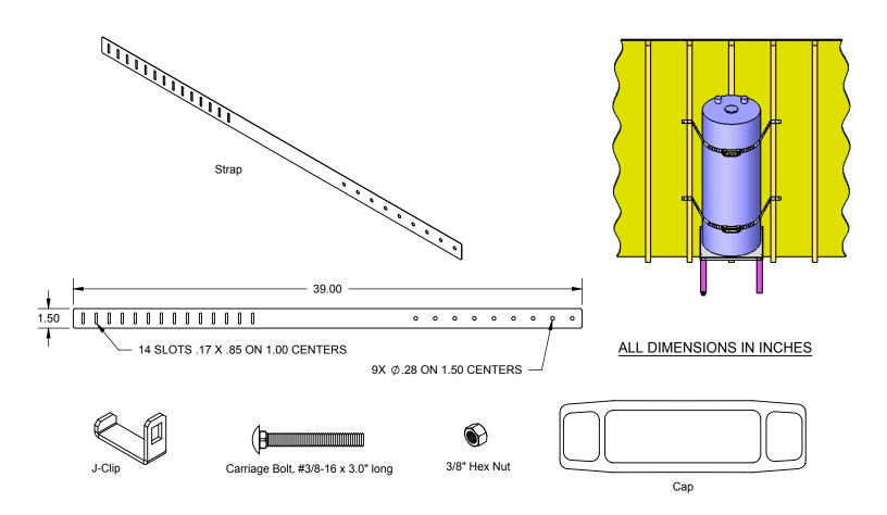
The QUICK STRAP® #QS-50-D is a seismic/earthquake support system for water heaters up to 80 gallons in size. The system includes: (4) Straps, (2) J-Clips, (2) 3/8" Carriage Bolts, (2) Caps and (2) 3/8" Hex Nuts. The Quick Link® system allows for full adjustment from the front side of the water heater.
