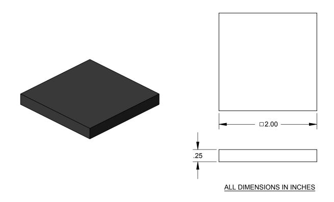
The HOLDRITE® Silencer™ #276 is an engineered sound and vibration isolation pad. Ideal for use in isolating riser clamps and equipment bases from noise transfer to the structure.
