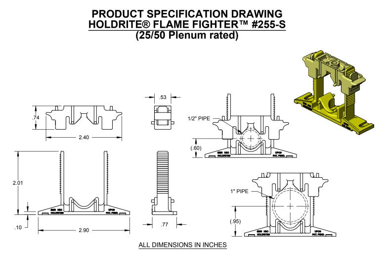
The HOLDRITE® Flame Fighter™ #255-S is a fire retardant and low smoke variable closure clamp that installs as a standard two hole pipe clamp with one or two screws. Clamp supports up to 1" CTS tubing sizes. Supports Copper, PEX, CPVC tubing, conduit, etc. Material meets ASTM E-84 25/50 and UL94V-0 fire rating.
