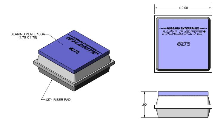
The HOLDRITE Silencer™ #275 is an engineered sound and vibration riser pad with a steel bearing plate. Ideal for use in isolating riser clamps and equipment bases from noise transfer to the structure.
