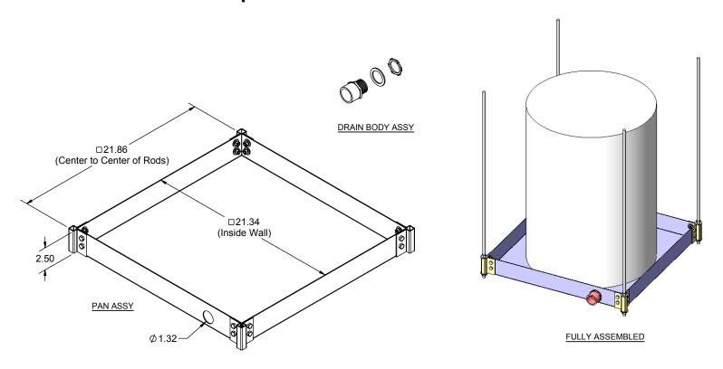
The Suspended Water Heater Platform is engineered to support water heaters up to 20 gallons (up to 375 pounds total weight). This time and labor savings tool is designed for the Professional Contractor. Design features requested by plumbers are incorporated into a professional platform that can be suspended with all thread rod.
