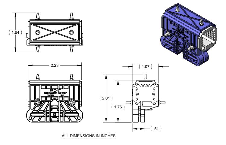
The HOLDRITE Silencer #265 Acoustical Shower Head/Tub Spout Clamp is a strong and effective clamp for minimizing the noise generated at the shower or similar application. This clamp is designed for attachment to the Holdrite Stout Bracket® and accepts a drop eared 90° ell or similar fitting.
