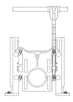
The HOLDRITE #114-C is a Copper-Bonded™ steel bracket with two slots for securely mounting upright to the carrier unit. The top end has a single 1-1/8" extruded hole for soldering 1" copper pipe, as well as supporting the water pipe for the flush valve above the floor. Adjust the flush valve 4-1/2" from the carrier center and 14" above the top fixture mounting bolt. This installation typically places the flush valve at 11-1/2" above the fixture, When soldering, heat the pipe, not the bracket.
