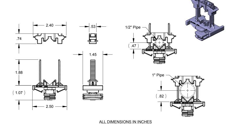
The HOLDRITE® Strut Clamp™ #257 is a strong variable closure clamp. Clamp supports up to 1" CTS tubing sizes. Supports Copper, PEX, CPVC tubing, conduit, etc. Framework complies with UL94V-2 fire rating.
