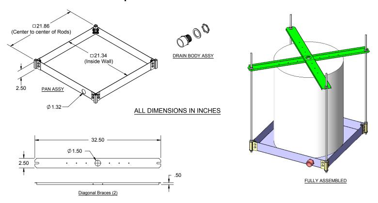
The Suspended Water Heater Platform is engineered to support water heaters up to 20 gallons (up to 375 pounds total weight). This time and labor savings tool is designed for the Professional Contractor. Design features requested by plumbers are incorporated into a professional platform that can be suspended with all thread rod.
