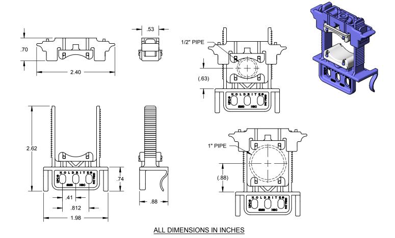
The HOLDRITE® Stout Clamp™ #250 is a strong, sound rated variable closure clamp compatible with Copper, PEX, CPVC pipe, conduit, etc. Supports up to 1" CTS tubing sizes. Frame work complies with UL94V-2 fire rating and UPC listed.
