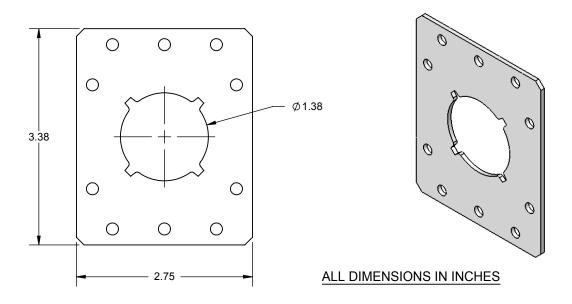
The PEXRITE® #721 is a 14 gage galvanized steel bracket that integrates directly with the PEXRITE® #701 Clamp, #704 Insert and HOLDRITE Stout Brackets®. It provides a PEX pipe support solution for lavatory and toilet applications. The #721 also attaches directly to wood, metal or concrete and various HOLDRITE® #100 and #400 series inserts.
