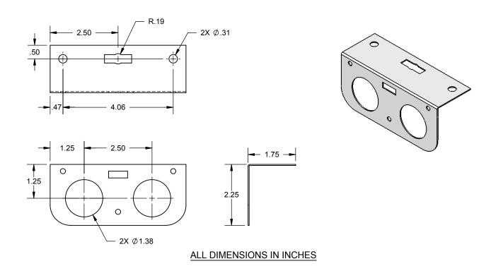
The HOLDRITE® #121-DS is a 20 gage galvanized steel bracket the supports dual lines of 1/2", 3/4" or 1" Copper, PEX or CPVC tubing at 1-1/4" center line height. The hole pattern on the 90° base allows for attachment to any flat surface. The bracket can also be suspended by 3/8" threaded rod.
