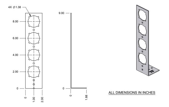
The PEXRITE® #709-EXT is a 14 gage galvanized steel bracket with 1-3/8" keyed holes providing a 2", 4", 6" and 8" center line off of the attachment surface. Designed to work with our PEXRITE® #701 Clamp and #704 Insert. Ideal for toilet water supply lines. Compatible with HOLDRITE® Silencer<sup>™</sup> #261 and #262 and with #100 and #400 series inserts.
