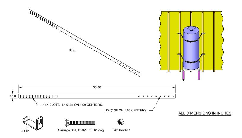
The QUICK STRAP® #QS-120 is a seismic/earthquake support system for water heaters up to 120 gallons in size. The system includes: (4) Straps, (2) J-Clips, (2) 3/8" Carriage Bolts and (2) 3/8" Hex Nuts. The Quick Link® system allows for full adjustment from the front side of the water heater.
