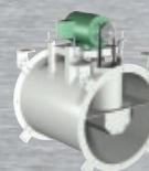
**Model TCB** inline belt driven fans are the ideal choice for installations with straight-through airflow in ducted systems. The wheels used are designed to provide higher efficiencies and lower sound levels. The fan itself can be mounted horizontally or vertically. Performance ranges up to 24,000 cfm (40,800 m<sup>3</sup>/hr) and up to 4.5 in. wg (1120 Pa) of static pressure.
