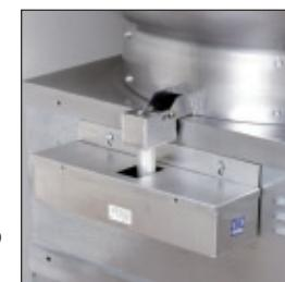
**Grease Trap** - Aluminum trap designed to collect grease residue to avoid drainage onto roof surface. (Roof Upblast only.)
