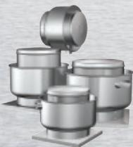
**Models CUE, CUBE, CW, and CWB**, Series C, are commonly used for general clean air, mild grease, and fume hood exhaust applications. Both Roof Upblast and Sidewall configurations are specifically designed to discharge air directly away from the mounting surface. These models are constructed of aluminum and use an aluminum backward inclined wheel. They are UL/cUL Listed for electrical or grease. Performance ranges up to 5 in. wg (1245 Pa) and up to 30,000 cfm (51,000 m<sup>3</sup>/hr).
