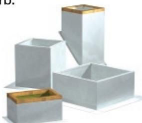
**Vented Curb Extensions** - Mounts between roof curb and roof mounted fan to meet NFPA requirements of 40 in. minimum discharge above the roof when mounted on a minimum 8 in. high roof curb.
