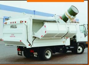
Eliminate lifting of barrels with optional barrel dumper.
