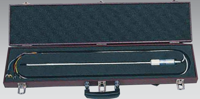
Super Stable Standard Platinum Resistance Thermometer
