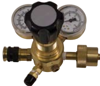
PAI-0002RA1 Single Low Pressure Regulator 3000 PSI / 204 BAR 5.5" x 5" x 4" (16.5 x 12.7 x 10.2 cm) 3 lbs (1.4 kg)
