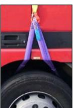
The suspension of modern truck cabins permit maximum joint travel and effectively balance out vibrations. During rescue work after an accident, any kind of movement may have a negative influence on the condition of the patient. Any movement made by an involved vehicle must be avoided to effectively remove the patient.
