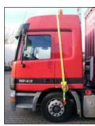
be hooked into holes in the wheel rims on both sides and tightened with a ratchet. A loop can also be laid around the front axle section.
