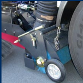
ABOVE Combivac nozzle enables higher sweeping speeds
