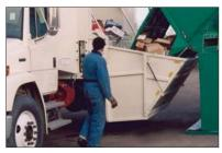
Service a Hyd-A-Way<sup>®</sup> container in under 3 minutes! Large bucket volume (up to 5 cu yds/ 3.8 cu m) minimizes loading time to optimize collection efficiency.
