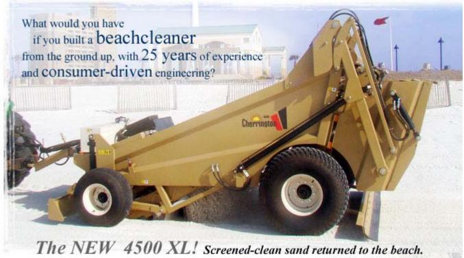
To thoroughly clean a beach you need to screen the sand, removing all the debris larger then the chosen screen hole size. Screening is the only way to not only completely clean the beach but aerates and conditions the sand, while also reducing bacteria and e-coli.
