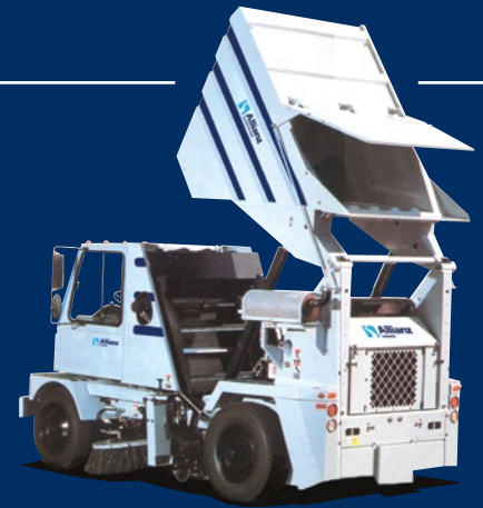
TOP 5.6 cu. yd. high dump hopper allows for longer sweeping distances before unloading.
