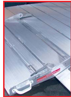
A 2,000 lb capacity, 72-inch Walco all aluminum cam closure liftgate with flip-out extension and cart stop
