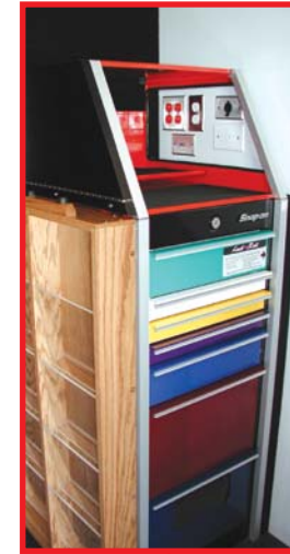
The mobile office features plenty of room for laptop computer, printer, sliding brochure rack, metal storage drawers, portable broken tool drawer, and formica flip-down writing surface for customer orders and receipts
