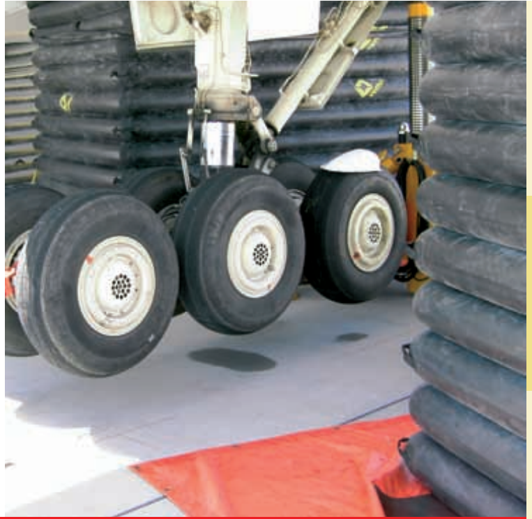
Aircraft Lifting Bags 1.0 bar/14.5 psi
