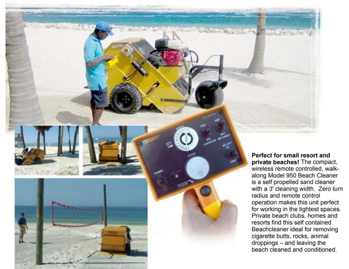
Easy joystick steering with independent rear wheel drive provides great maneuverability in confined areas. The 950 can safely work within inches of walls, trees and cabanas. The 950 Sand Cleaner also works great on volleyball courts, ball fields, small resort beaches and even firing ranges. The wireless remote control lets the operator control the operation of the 950 from a distance through, around, and underneath beach and playground enhancements.
