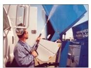
Collection vehicles with an onboard **pressure** washer keeps containers sanitized & odorless.
