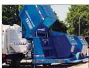
Transfers material into MRF drop off bins for ease of operation and greater convenience.
