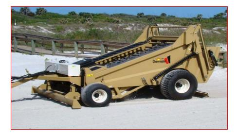
Cherrington uses a new advanced engineered hydraulic system to power a sifting screen so intensely that it makes for fast routine cleaning and deep down Beach Sanitizing. Carbide glide pucks for long life, and a smooth, quiet, operation.
