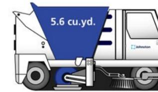
**7** Dirt conveying system is hydraulically opened from within the cab to ingest bulky debris such as branches and leaves. Three dedicated hydraulic pumps provide maximum sweeping power to the gutter broom, pick-up broom and dirt conveying system. Dirt conveyor features an overthrow system for quick debris transfer and maximum hopper loading capacity.
