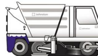
**6** 5.6 cubic yard hopper versus 3.5 cu. yd. for competitive machines, dramatically increases curb miles swept between dump cycles. Constructed entirely of stainless steel and covered by a lifetime warranty, ensuring the lowest cost of ownership and guaranteeing greater re-sale value.
