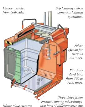
Lifting plate ensures bin wheels are not damaged.
