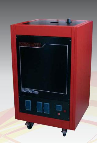
Fixed Points of: Indium 156.5985°C, Tin 231.928°C, Zinc 419.527°C, and Aluminium 660.323°C Active and Passive Safety Circuits, Equalizing Block for Comparison Calibration
