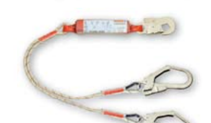
PRO™ LANYARD 1.8m double-leg shock absorbing lanyard with 10.5mm kernmantle rope and steel scaffold hook ends with 50mm opening. AE532/3
