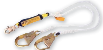
SHOCKWAVE2™ LANYARD 6 ft. (1.8m) double-leg 5/8" (15.8mm) rope shock absorbing lanyard with aluminum rebar hook ends with 2-1/4" (57mm) gate opening. 1246001 (Not Available in Canada)
