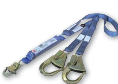
HEAVY DUTY LANYARD Twin-tail lanyard for heavy duty applications where the combined body weight of the user is up to 160kg. 2m length. 60mm opening scaffold hooks. Z60201819H
