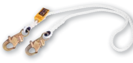
ROPE POSITIONING LANYARD 6 ft. (1.8m) single-leg positioning lanyard with 1/2" (12.7mm) nylon rope and standard snap hook ends with 3/4" (19mm) opening. 1232354 (1220361C - 5/8" rope in Canada)
