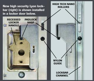
Nano rollers ride effortlessly up the door jambs and drop into place, providing up to three and one half times the resistance to break-ins compared to other locker latching systems. (Note: for demonstration purposes, top nano roller has been lowered into close proximity with locker handle.) New nylon lockbar guide ensures lockbar alignment and eliminates metal-to-metal contact.
